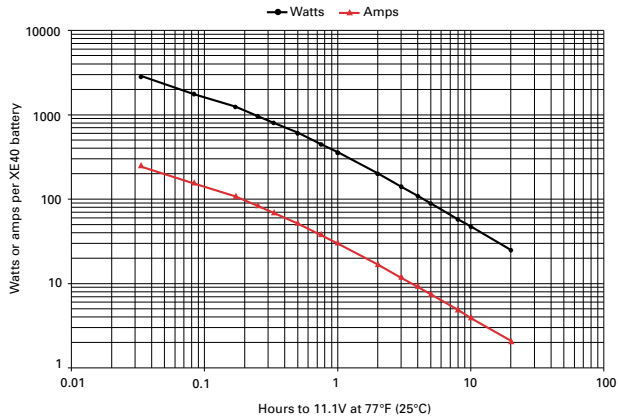
Figure A-16: XE40 discharge data to 11.1V at 77°F (25°C)
