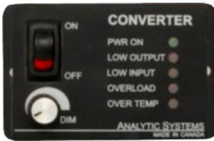
A remote control panel may be connected to the converter using a 9-pin D-connector, which attaches to the front panel of the voltage converter. The remote control panel and D connector are part of the remote control option. The remote control panel allows the unit to be operated remotely as well as duplicating all the diagnostic indicators and audible alarm.
